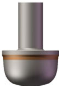
Partial welding on sealing face of plug
